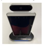
Step 10: To adjust tablet tilt—loosen top nut behind tablet on post then adjust to desired location and retighten nut
